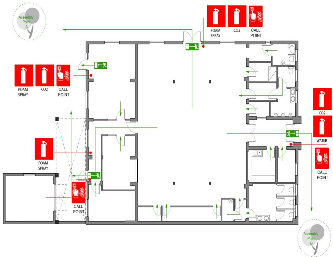
FIRE EXTINGUISHER & CALL POINT LOCATIONS
