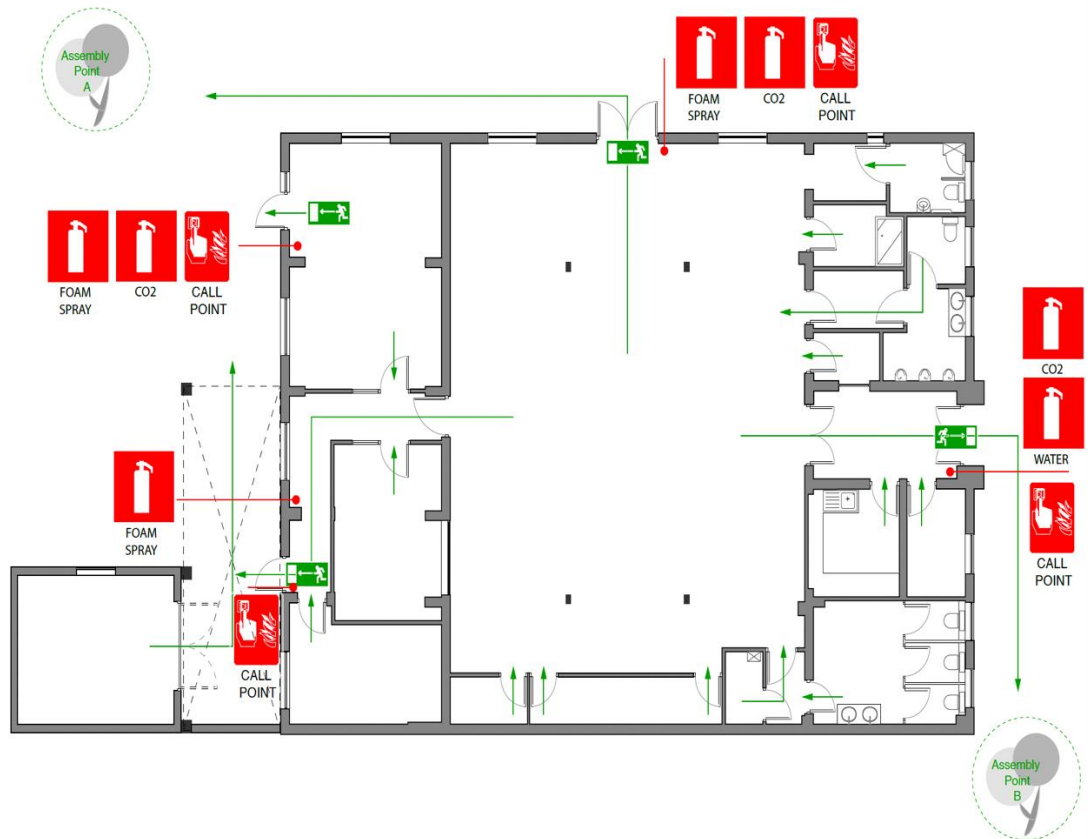
FIRE EXTINGUISHER & CALL POINT LOCATIONS
